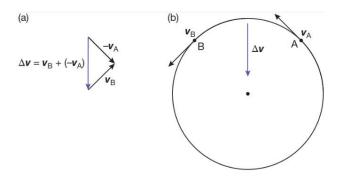
As the object is moving with uniform circular motion, the lengths of the vectors  $v_B$  and  $-v_A$  are identical (both equal to the object's average speed v) and so form two sides of an isosceles triangle as shown
