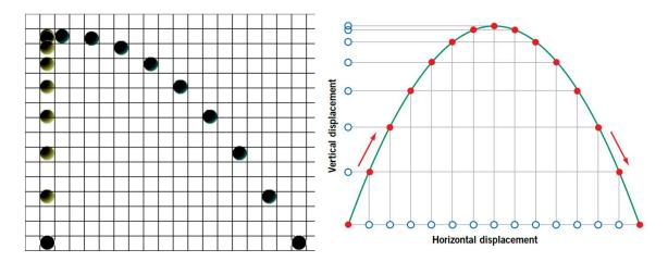
Since the projectile moves the same horizontal distance every time, its horizontal component of velocity must be constant.  $s_x = u_x t$ .
