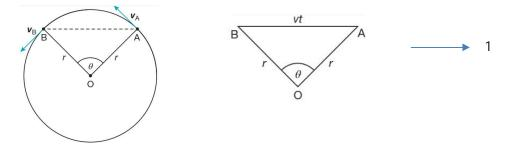
OAB is seen to form an isosceles triangle with OA = OB. The third side is formed by a line, or chord, joining A with B. When the angle  $\theta$  is small, the length of this chord is virtually the same as the length of the arc which also joins these two points. As this distance is covered by an object travelling with an average speed v in a time t, the length of AB can be calculated using s = v t.
