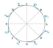
If a body moves with constant speed 'v', in a circle of fixed radius 'r', its velocity 'v' at any point has magnitude 'v' and is directed at a tangent to the circle at that point.
